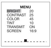
Press **MENU** button repeatedly to select among BRIGHT, CONTRAST, COLOR and TINT (For the unit with NTSC system) items and etc. Press **VOL+/VOL**buttons on the unit or **VOLUME** +/-buttons on the remote control to adjust the corresponding item.
